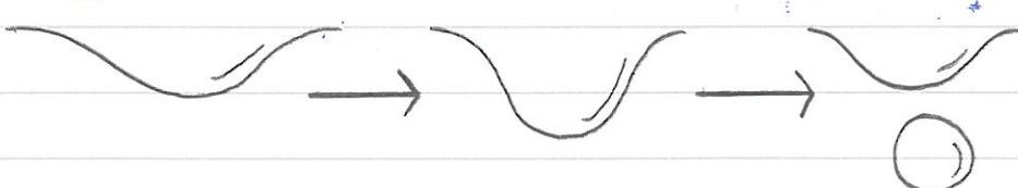
This happens when surface tension is no longer a match for gravity. Let us make a very simple model of the drip as a cylinder of water.
